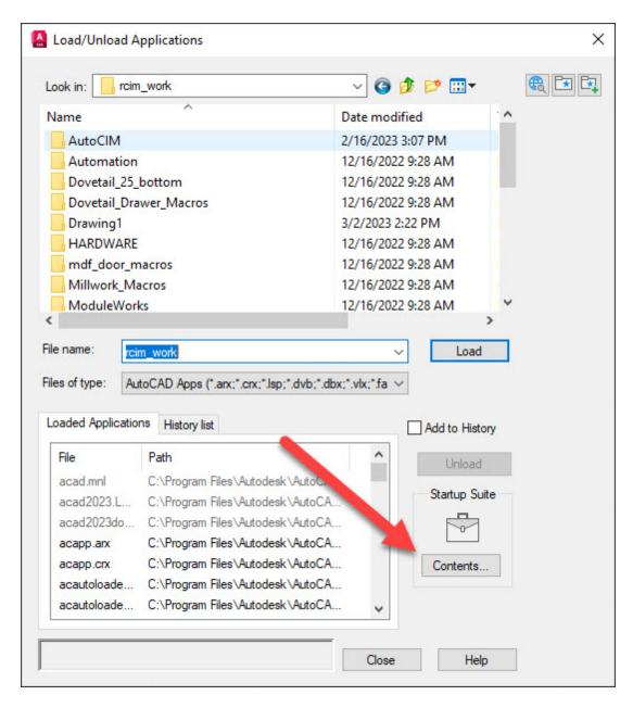
Click on the Startup Suite Contents in the lower right corner and add the new routine into the contents of the Startup Suite.
