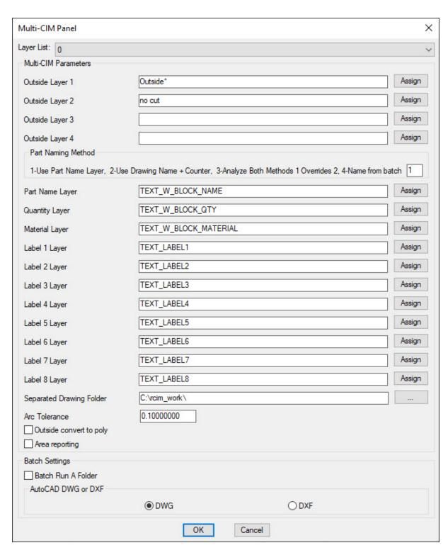
From here you can set the name of the layers that contain your Outside Geometry. There is a pull down list at the top so that you can check the names and spelling of the layers to add to the lists.
