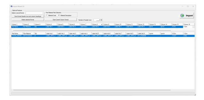
Pull down the column header that says **Select Data Type** above each row and set them to the correct fields. The first one is the **Part Name**, the second is the **Part Material** and the third is the **Quantity** (**Qty**).
