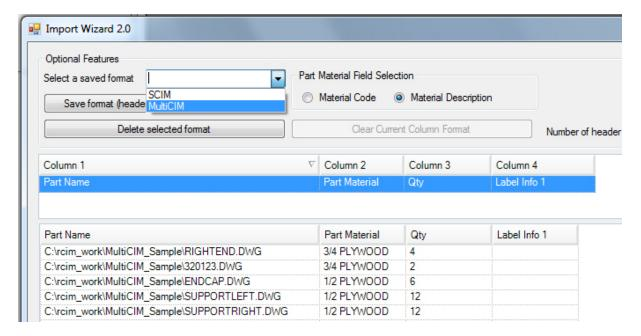
Once the columns have been assigned or a saved format has been applied, select the **'Import'** button and a job will be created in Router-CIM Automation Suite.
