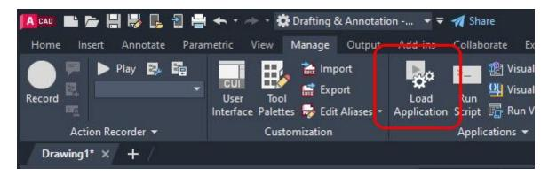
A new window will appear where you can set the Start Up routines you want to run when AutoCAD starts up.
